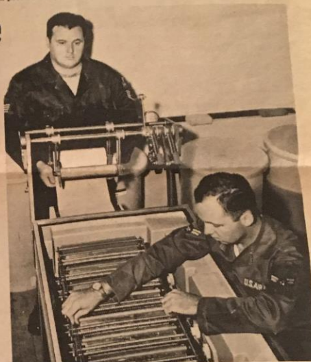
FILM PROCESSING—SSgt. Larence Dow (left) and A2C David Reed operate the versamat processing machine in the Photo Lab Branch, used for processing aerial photographic film.
